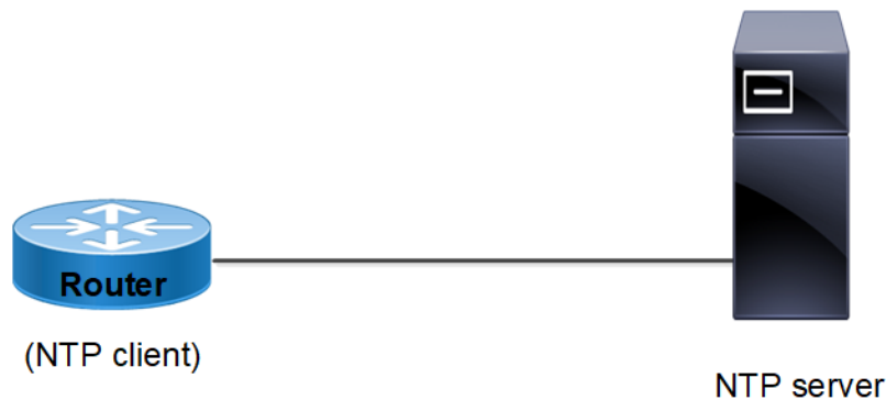
Figure 32. NTP Client topology
