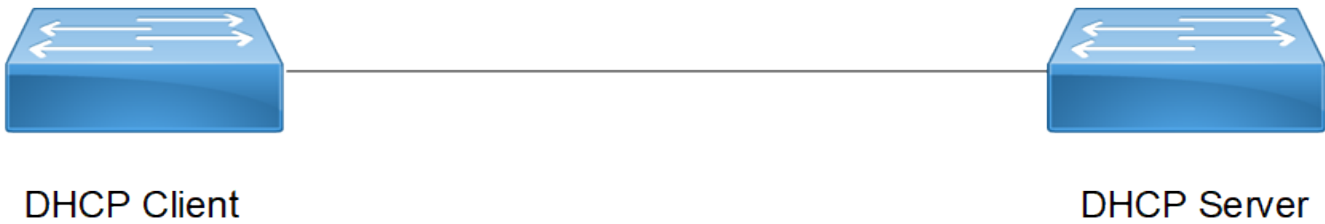
Figure 27. DHCP IPv4 topology
